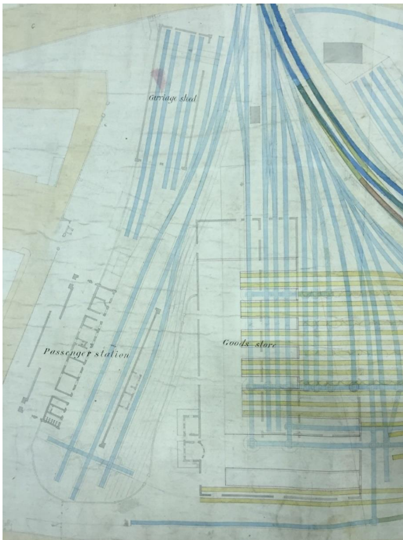
Figure 3: This drawing, taken from the collection of the Irish Railway Records Society, shows the complex arrangement of tracks running into the three buildings on the site: the large number of tracks running into the Goods Shed indicates its importance in transporting large goods by rail
